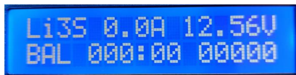
Figure 8. Now the battery is charging. Press Stop (red text) to stop charging. (NOTE: Always stop charging before unplugging the cables.)
