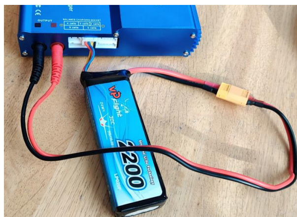
Figure 4. This is what it looks like if the battery is connected correctly. (NOTE: Never charge the battery without being in a charging bag.)
