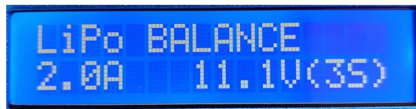
Figure 5. Make sure the charger is in BALANCE mode. Change mode by pressing Inc. or Dec. the buttons. Then hold down the Start button until the charger beeps to start charging.
