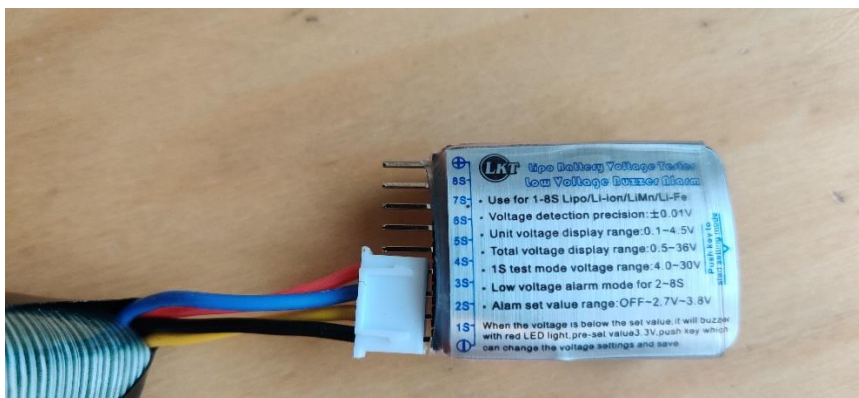
Figure 1. This is how to connect the alarm to the battery. (Tips: The alarm beeps loudly when connected, so block the speaker with a finger when connecting it and it will not beep as loud.)
