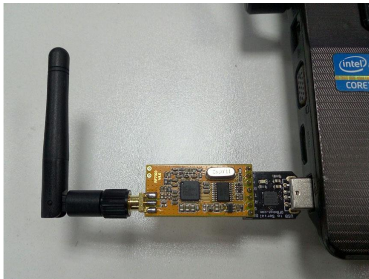
Figure 1. The radio module with a bent pin plugged in via a USB-UART adapter.
