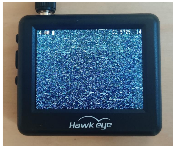
Figure 1. Camera receiver set to 5725 MHz. The letter C shows that the receiver is set to frequency band A, which is used by all the team's cameras.
