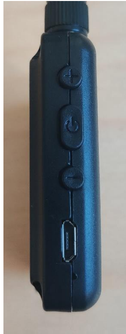
Figure 2. Camera receiver with power button in the middle, plus button to change the frequency band and minus button to change the frequency within the selected band.
